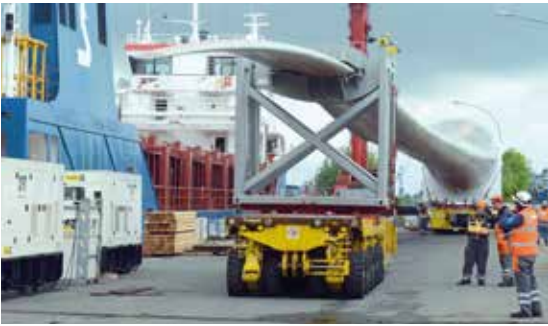
Transport of a rotor blade prototype (83.5 m Length, 34 t weight) with 2x 6 axles
