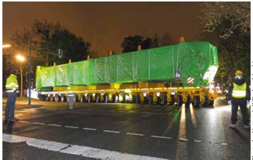
Transport of modules for a power plant (194 t) with 1x 18 axles
