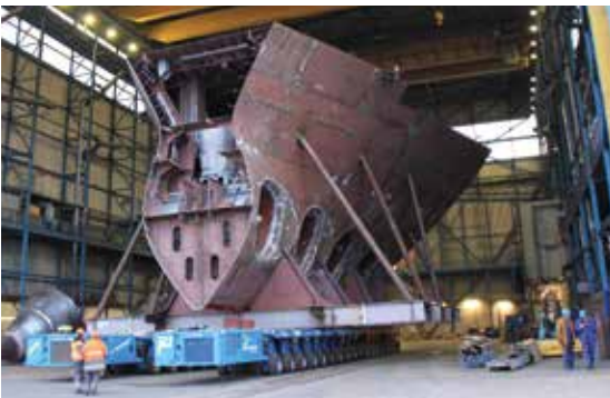
Transport of a ship section (280 t) with 2x 18 axles
