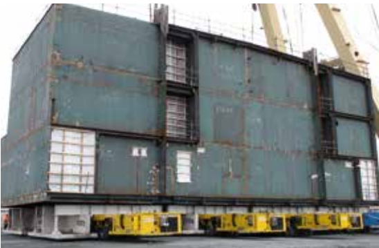
Transport of an offshore topside section weighing 1,200 t with 4x 12 axles
