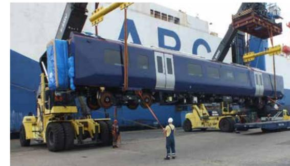
Handling of railway waggons ex/on truck, trailer or railtrack.
