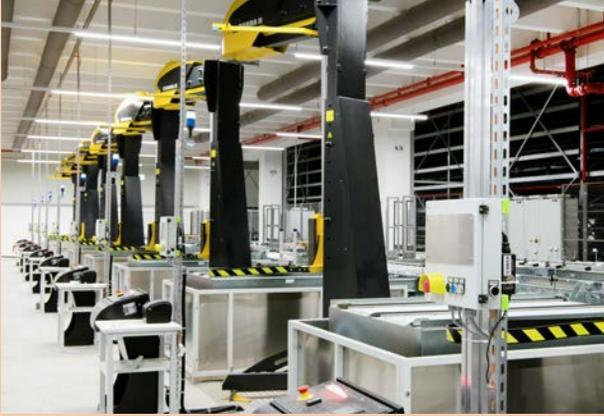
**Top:** The result is a highly automated warehouse with 22 kilometers of conveyor technology and 480 shuttle vehicles.
